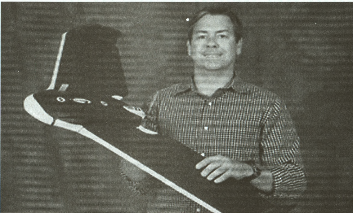
Michael Starek holds the SenseFly eBee, a fixed wing platform that acts like a miniature plane.
