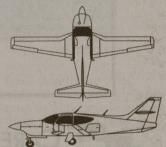
Accommodation: Four (including pilot) Wing span: 35 ft., 7.4 in. Lenght: 24 ft., 10 in. Heigh: 8 ft., 5 in. Max. speed: 170 mph
