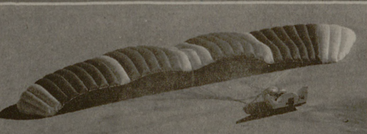
The world's largest parafoil slowly deflates after carrying the X-38 to a safe landing. Photo Courtesy: NASA
