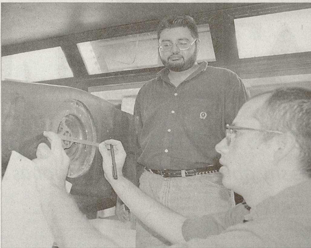
Khurram Rehmatullah and Carlos Yapura, research associates at the Texas A&M low-speed wind tunnel, prepare a model of NASA's new X-38 space shuttle for aerodynamics testing.
