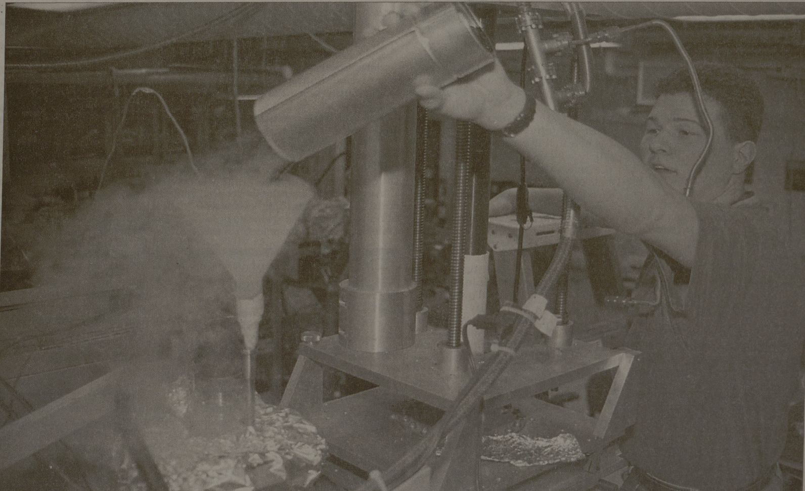
Doug Meier , a chemistry graduate student, adds liquid nitrogen to an ultra-high vacuum chamber. The low-temperature liquid helps improve the vacuum, which is used to test metal catalysts.
