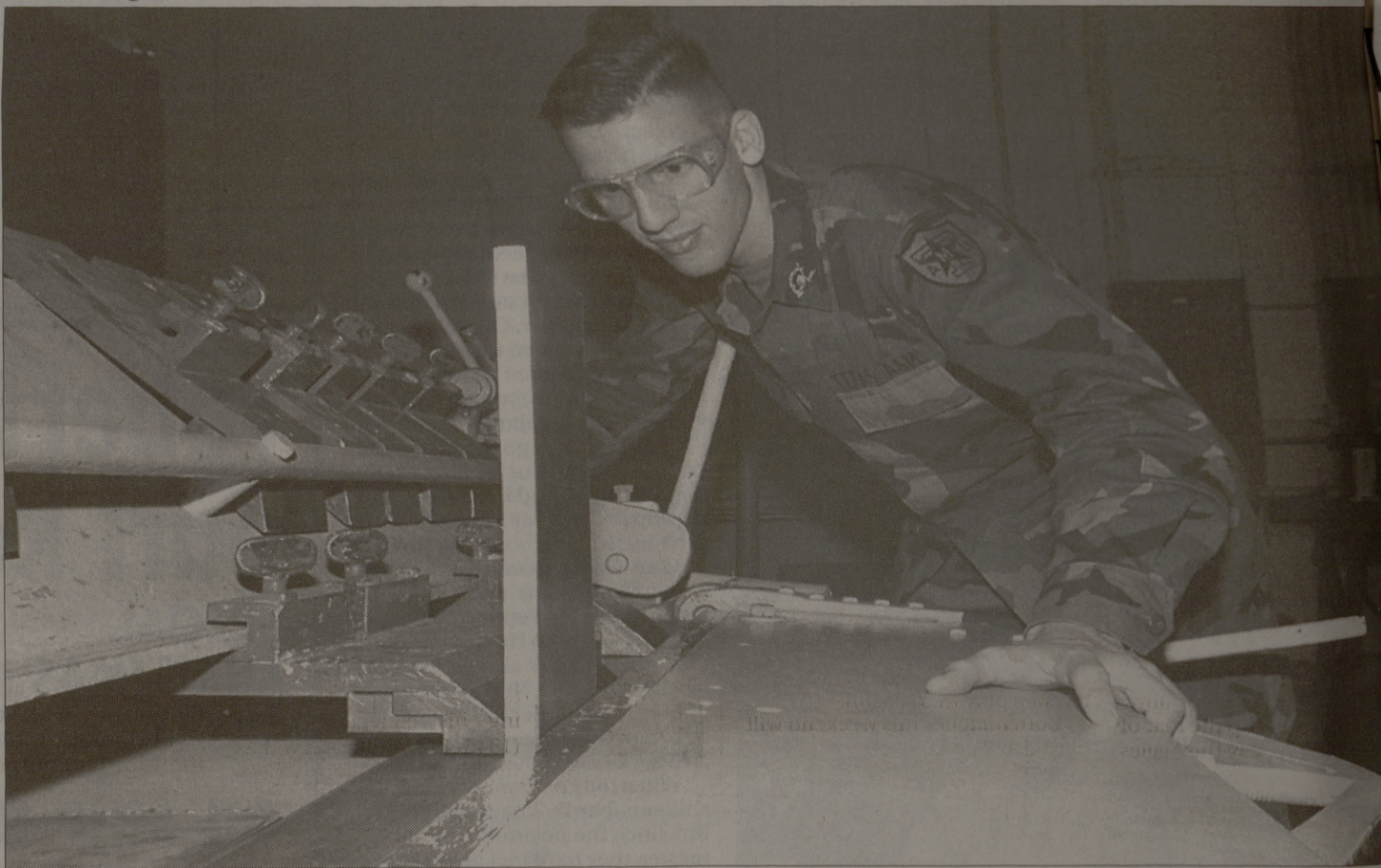
Max Mondelli, a junior mechanical engineering major, bends sheet metal to form a box lid in an Engineering Technology 181 lab Thursday afternoon in Thompson Hall.
