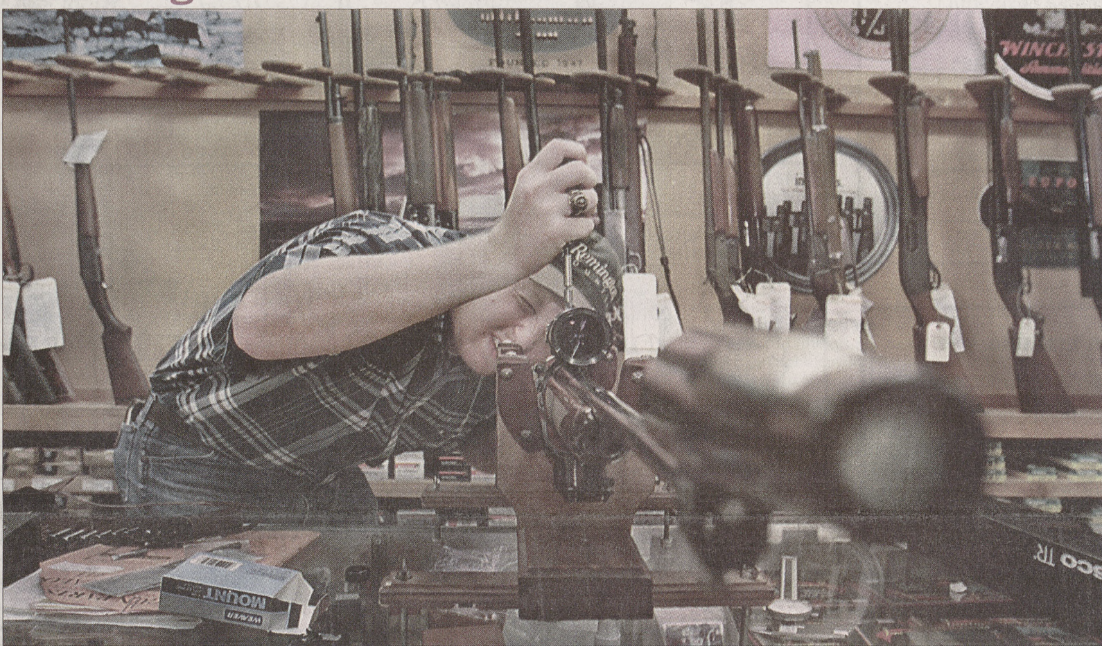
Mike Mizzell, a senior agriculture economics major, mounts and bores a telescope sight for a customer at Sullivan's Outfitters Monday afternoon.
