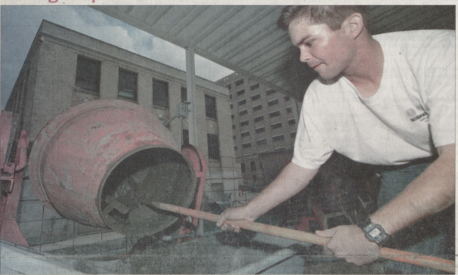
Jeff Heffington, a senior Civil Engineering student, mixes concrete in his Civil Engineering 342 class. The students make test beams and columns which they then test for strength.
