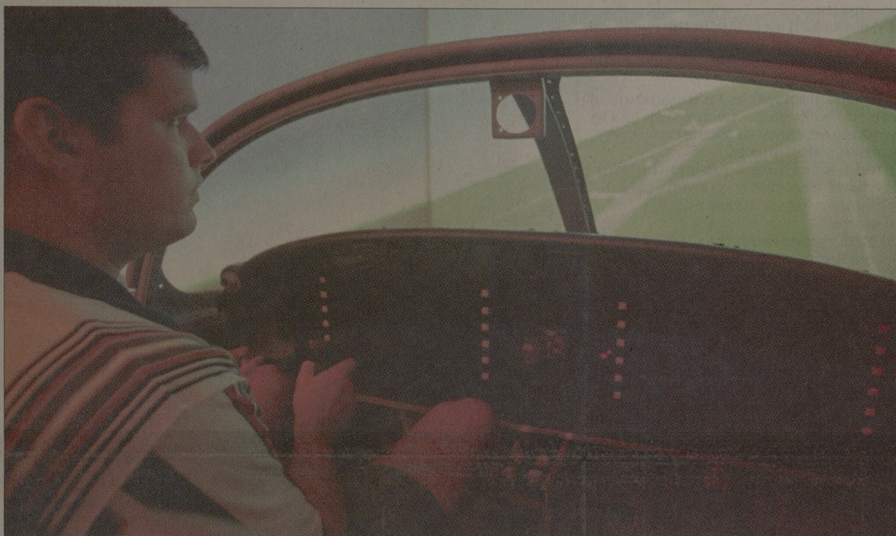
PHOTOGRAPH: Shannon Castle Drew Robbins, a graduate aerospace engineering student, operates the 'smart cockpit' flight simulator in the Bright Building. The simulator is made from a T-37 fuselage.
