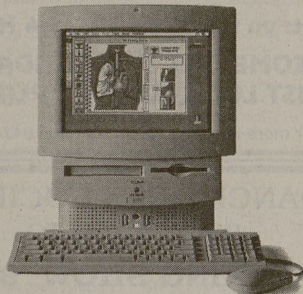
Macintosh® LC 575 5/160, internal AppleCD™ 300i Plus CD-ROM Drive, Apple® Keyboard II and mouse.
