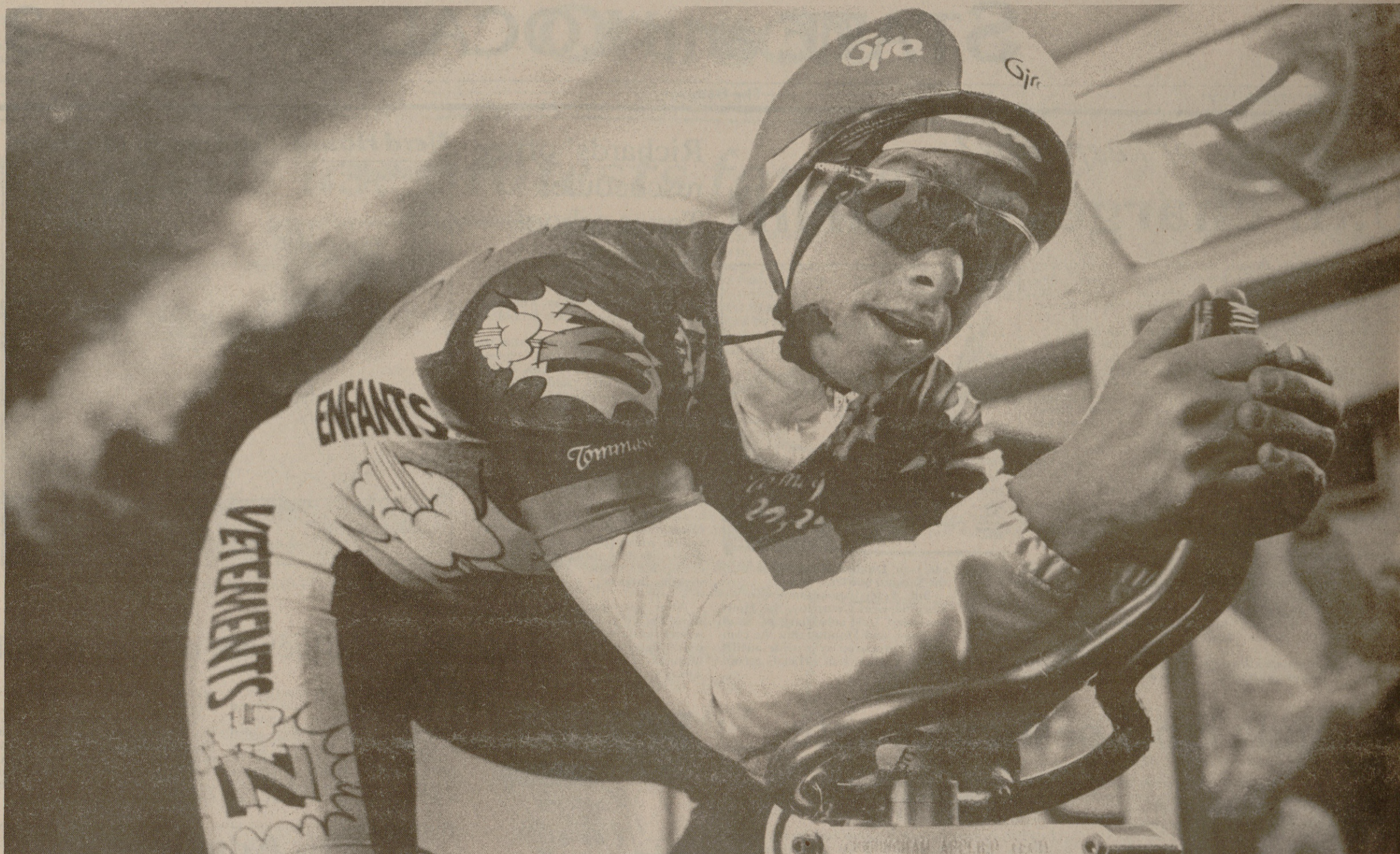
Smoke streams over LeMond's head to give engineer a 'look' at the air-flow.
