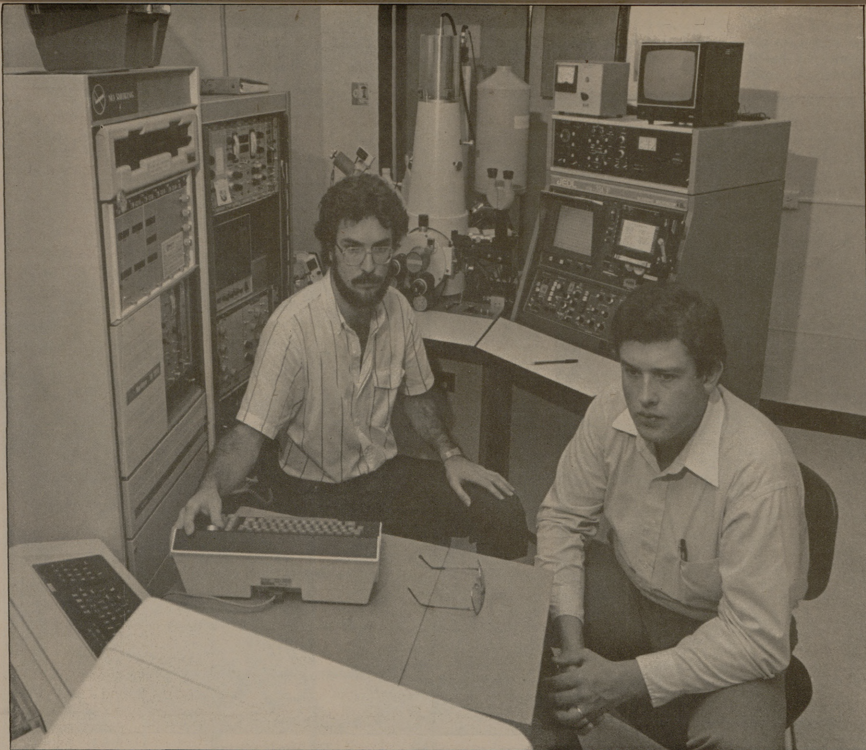
Jim Ehrman and Alan Huffman use a scanning electron microscope fitted with an X-ray attachment to analyze the elemental content of a mineral sample. Ehrman is a research associate with the Electron Microscopy Center at A&M and Huffman is a graduate student in geophysics.
