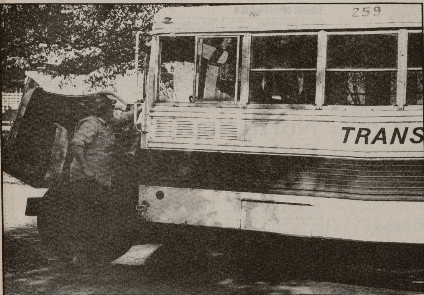
Bruce Walston, of Transportation Enterprise Inc., replaces a broken hose in this shuttle bus. The hose, which carried coolant to the engine, was punctured and caused the engine to overheat.
