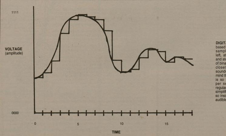
**DIGITAL RECORDING** is based on a system which samples a sound wave, left, at a very rapid pace, and stores on tape a series of binary numbers that very closely approximate the soundwave curve. Keep in mind that the sampling rate is so high (about 40,000 per second) that the irregularities that exist in this simplified drawing become so insignificant as to be inaudible to the human ear.
