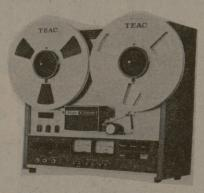
FORMAT: 1/4-track, 2-channel stereo HEADS: 3 (erase, record, playback). REEL SIZE: Up to 10½". TAPE SPEED: 7½, 3¾ ips ( 0.5%).
