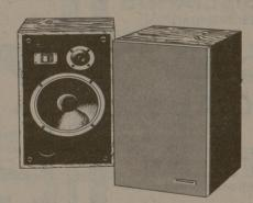
3-WAY 3-SPEAKER SYSTEM Enclosure: Bass reflex type Speakers: 10-inch carbon fiber blended cone woofer, 12%z-inch carbon fiber blended cone tweeter. High-molecular polymer super-tweeter Impedance: 8 ohms Frequency Range: 35—25,000Hz Sensitivity: 91dB/W/ M Maximum Input Power: 40W Crossover Frequencies: 4,000 Hz, 10,000Hz Dimensions: 121%e"(W)×22%e"(H)×12½"(D)
