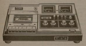
High Fidelity Stereo Cassette Deck with Dolby. HPF<sup>100</sup> head. Tape-End Alert-Eye. Peak check VU meters. CrO<sub>2</sub>/Normal tape selector. Separate mic/line level controls. Electronically controlled DC motor. Memory rewind. Mic mixing with separate volume controls for optional mics. Two muting circuits. Full Auto-Stop mechanism. Low-noise transistor circuitry and 2-stage direct-coupling.
