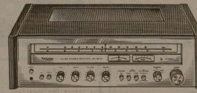
FM/AM stereo receiver. 35 watts per channel, minimum RMS at 8 ohms, from 20~20,000 Hz, with no more than 0.3% total harmonic distortion. Pure-complementary OCL power amplifier with current-mirror loaded differential initial stage. Two 10,000 µF electrolytic capacitors. Direct-coupled low-noise phono equalizer. MOS FET FM front end. Two tuning meters. Flat group delay filters in FM IF. PLL in FM MPX section. Tape 1→tape 2 dubbing. Simulated wood cabinet.
