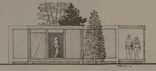
The units are concrete in construction and have the sturdy characteristics of permanent construction yet may be moved with little more difficulty than a mobile home. Each unit comes complete with heating, air conditioning, stove, refrigerator and carpeting. (The unit does not include furniture as illustrated.)
