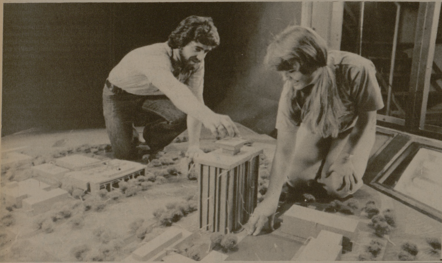
The TAMU wind tunnel, the bailiwick of aeronautical engineers, is being used to test the effect of campus buildings on the university environment. The large buildings apparently modify the prevailing winds and cause unusual phenomena. Vicki Moen adjusts a pitot tube at the base of the Oceanography and Meteorology Building while Steve Jones gives directions from behind the new architecture building.
