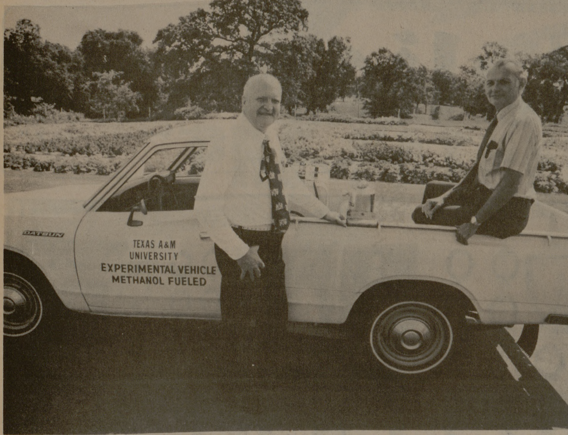
Drs. Bill Harris (left) and Dick Davison of TAMU have developed an auto conversion kit that allows them to start the car with gas then switch in a few miles to methanol which can be made from renewable resources such as garbage, sawdust, or any organic material and can also be conveniently made from coal. This solves problems previously associated with methanol use in conventional cars. The flowers in the background symbolize the fact that it is an extremely clean fuel that burns without smoke. See story page 1
