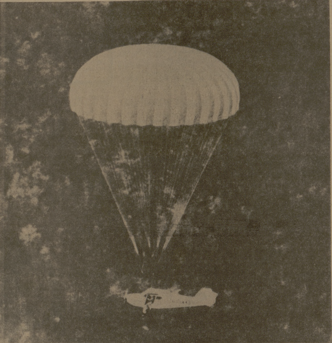
A LARGE PARACHUTE lowers a four-seat airplane safely to earth after the plane's wings were blown off. The incident was a test of a device invented by Dario Manfredi and Angelo Raiti. The men say they are still trying to market their safety system and have received no action on their 1967 request that the Federal Aviation Administration fund a study to apply it to use in heavier craft. (AP Wirephoto)
