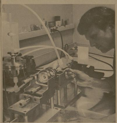
CONTINUOUS OUTPUT LASER using organic dyes has been developed by Kodak laboratories. The laser, which consists of a solution of yellow organic dye excited by an argon ion laser, is supposed to lower the cost of lasers as compared to rubies, glasses, and gases.
