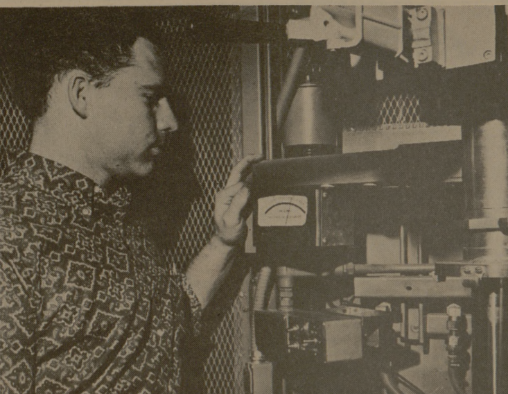
CYCLOTRON VACUUM CHECK Acceleration of particles in Texas A&M's cyclotron requires the machine be evacuated of virtually all air molecules. The cyclotron vacuum system is the responsibility of a crew of technicians, which includes Harry M. Elmendorf of Houston, who received Air Force training on pumping equipment. He checks a vacuum gauge directly under the accelerator chamber. Stainless steel pipe (right) is part of the accelerator's ion source.
