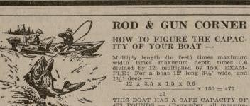
HOW TO FIGURE THE CAPAC-ITY OF YOUR BOAT — Multiply length (in feet) times maximum width times maximum depth times 0.6 divided by 12, multiplied by 150, EXAM-PLE: For a boat 12' long  $3\frac{1}{2}$ ' wide, and  $1\frac{1}{2}$ ' depth of the second se
