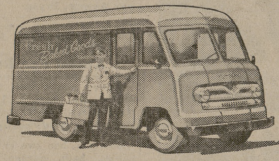
P-350 Parcel Delivery handles bodies up to 450 cu. ft. capacity. Fordomatic Drive, power brakes available.
