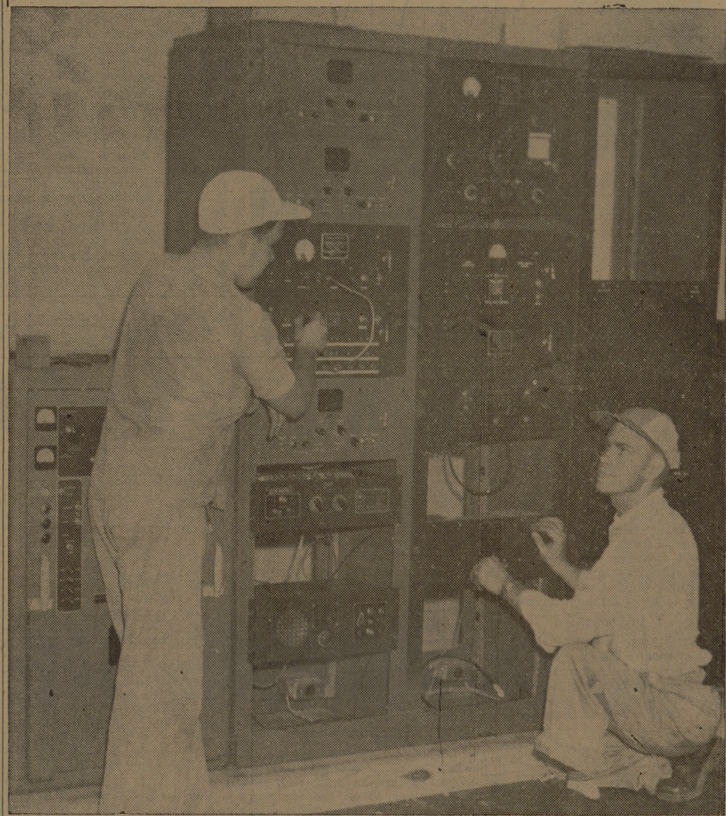
Adjusting the series of transmitters and receivers at the CAA Communications Station at Easterwood Airport which enables the station to keep radio contact with airplanes in the area are E. M. Gonzales, standing, and J. W. Philpot. Both are electronic engineers from Fort Worth.
