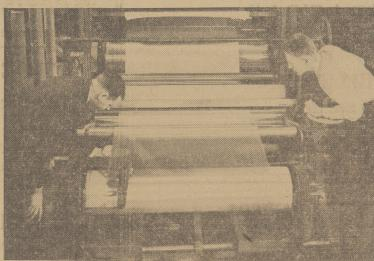
. M. Griffing, Ph.D. (Organic), Columbia '45, and A. Descheemaeker, B.S. in Chemical Engineering Lehigh'41, inspect PMA size solution and check nylon warp at head end of a slasher. In slasher sizing, entire warp is coated rather than a single thread.
