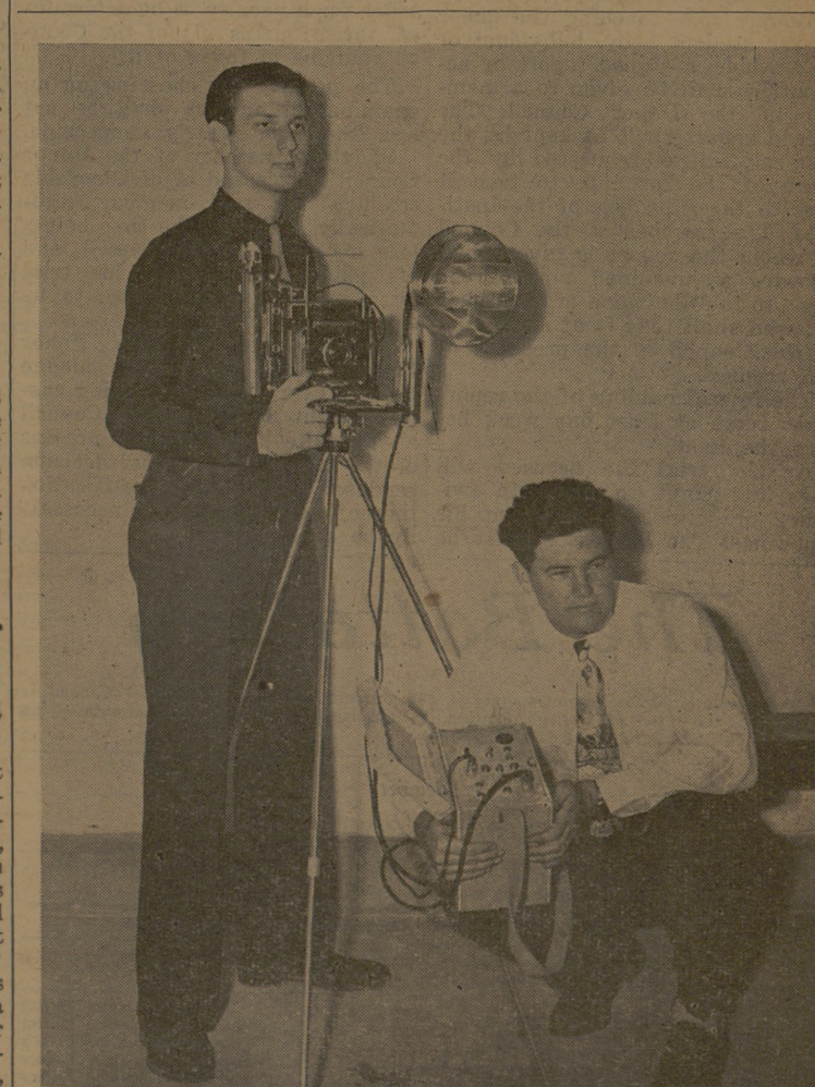
T. G. GRIFFIN (left) and CLAUDE R. STONE of the A. & M. Camera Club demonstrate the "stroblight" electronic device which goes away with flash bulbs. The apparatus, constructed by Griffin, releases a high-voltage impulse through a special lamp. The light produced is bright enough and fast enough to take clear photographs.
